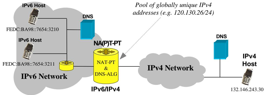
Figure 8 The use of NA(P)T-PT in an IPv6 network.
