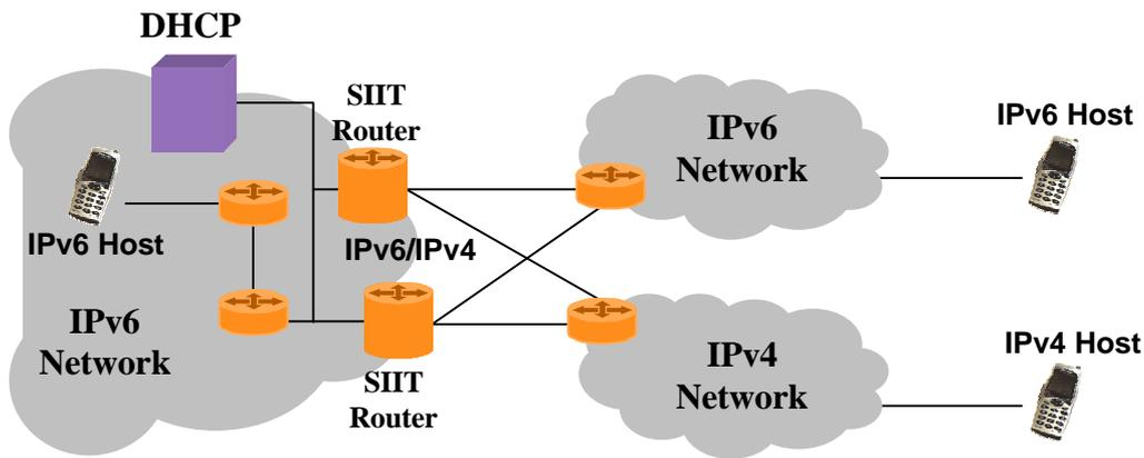
Figure 6 The use of SIIT within an IPv6 network
