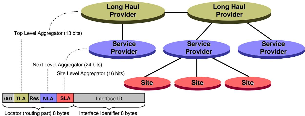
Figure 1 IPv6 unicast address allocation allows efficient route aggregation
