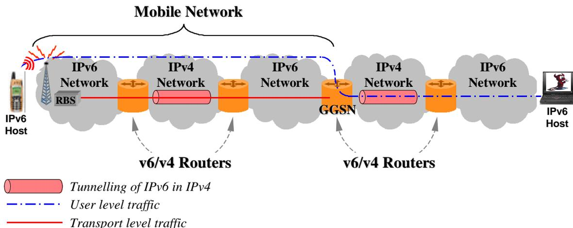
Figure 5 Connection of IPv6 sites via IPv4 networks
