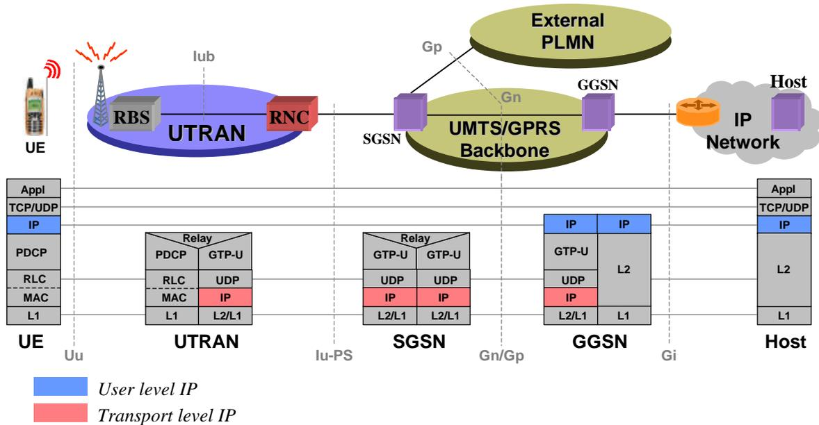
Figure 2 The 3GPP UMTS protocol stack illustrating the two separate IP layers
